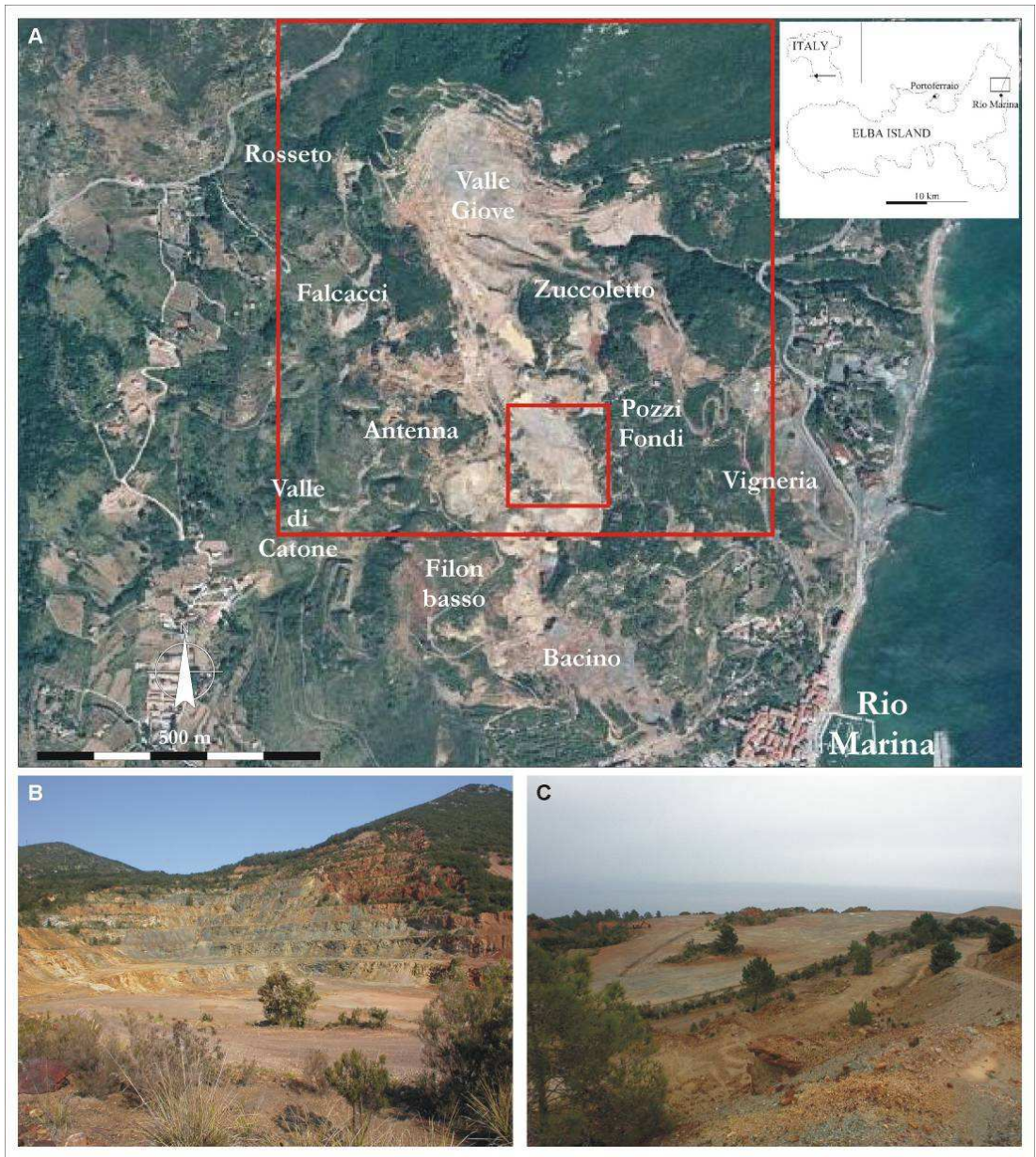
Fig. 7 - a) Aerial view of Rio Marina mining district (modified after Live Search Map, 2007 ). Names correspond to different mining sites exploited during the activity of mining district. The smaller red square identify the mine dump investigated with 2D-ERGI methodology, the bigger red square identify the boundary of the investigated area b) Valle Giove open pit, c) Antenna and Zuccoletto mine dumps
