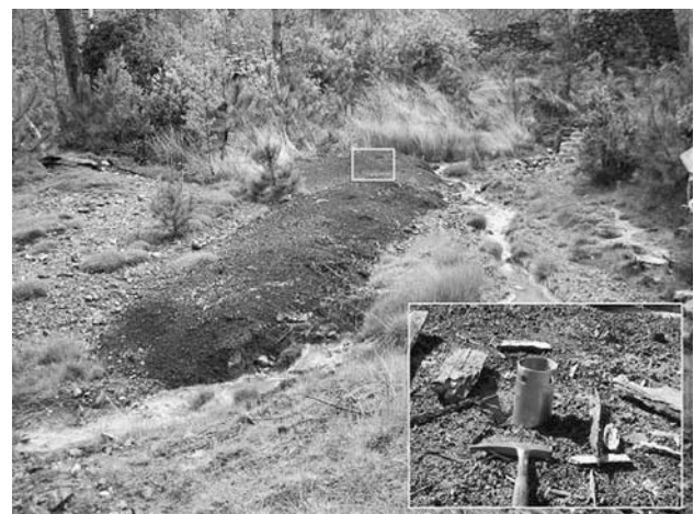
Fig. 4 Scenic view of the sampled tailing dump (TA); the white square and inset show the sampling area of the TA1 core
