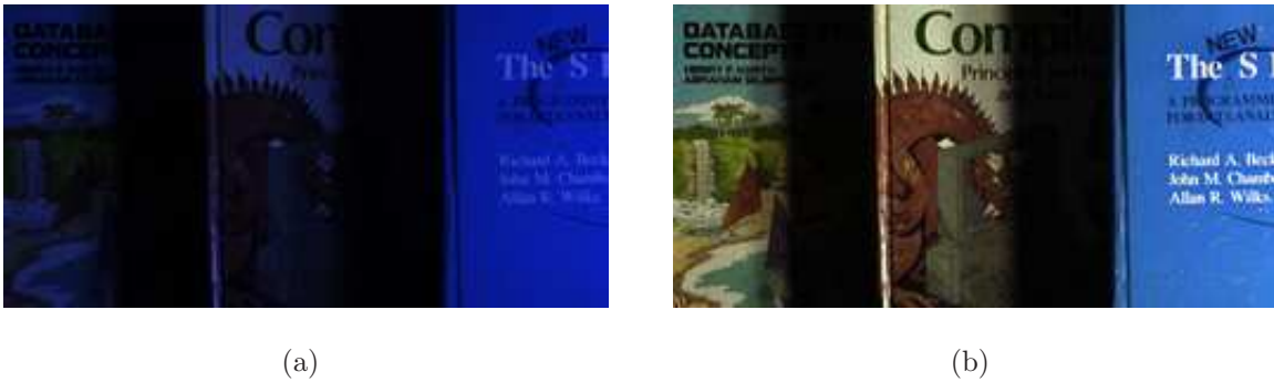
Figure 3.25: (a) Original "Books" image; (b) "Books" filtered with tuned parameter N = 25 , n = 750 .
