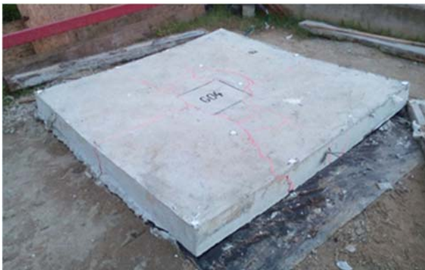
Fig. 2: Concrete slab - after the test
