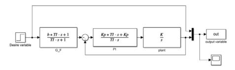
Fig. 3 Simulation scheme
