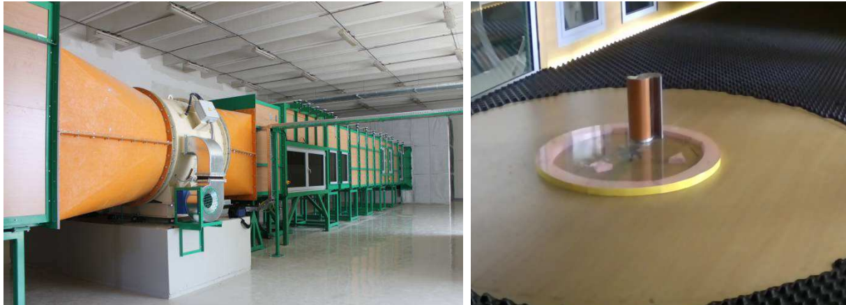
Fig. 2: The wind tunnel - BLWT STU and the experimental "S" model [6].
