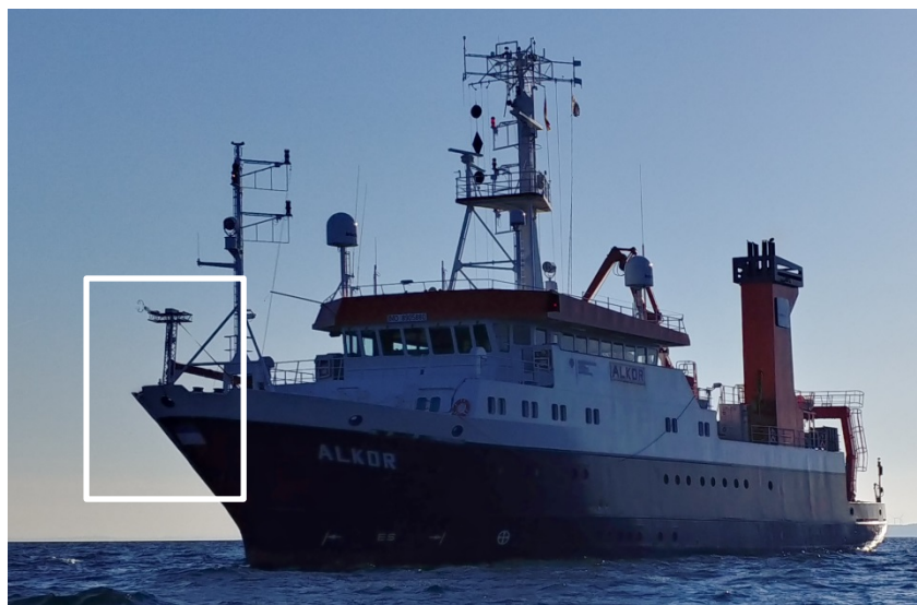
Figure 6: Mast including sensors and air inlet at the bow of the Alkor.
