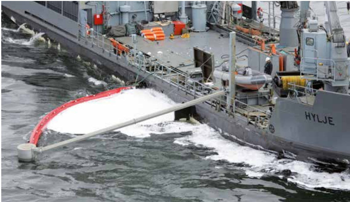
1.45 > During an oil spill exercise off Helsinki, the multipurpose vessel Hylje uses a sweeping arm to capture foam that is specially designed to simulate an oil slick.
