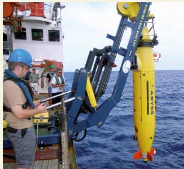
2.30 > A research ship crew member deploys an autonomous underwater vehicle (AUV) equipped with sensors into the sea.
