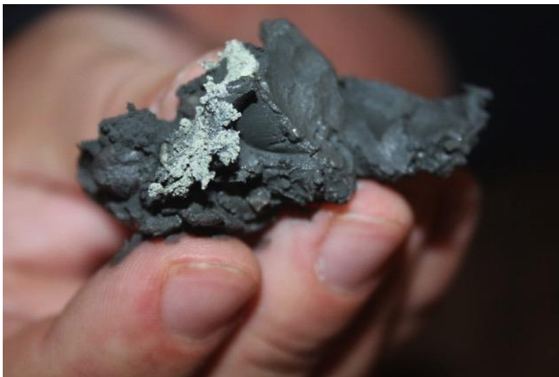
Figure 9: Disseminated carbonates from the core catcher of MSM78-11-20.
