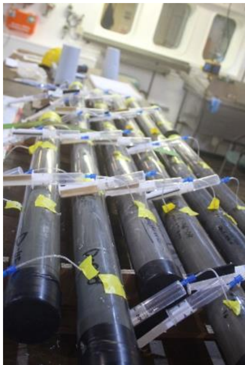
Figure 8: Porewater subsampling from gravity cores with Rhizones.
