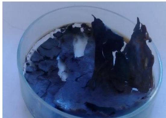
Figure 15: BCC composite membrane with an optimum concentration of PS clay of 8% (w/v).
