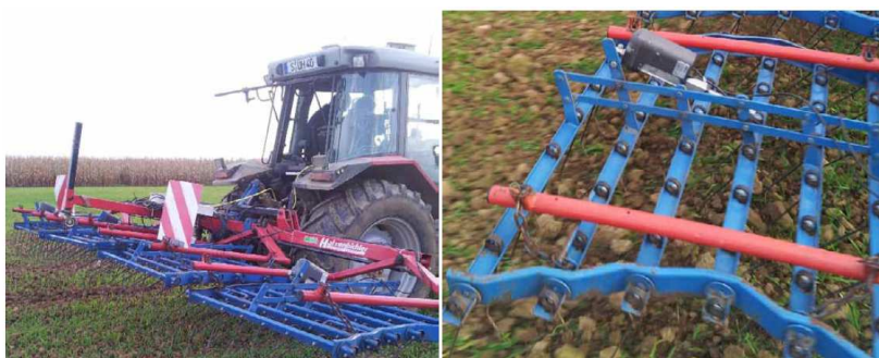
Figure 41: The flexible-tine harrow designed by Peteinatos et al. (2015). Left: the full tine with its four actuators. Right: Detail of one actuator.
