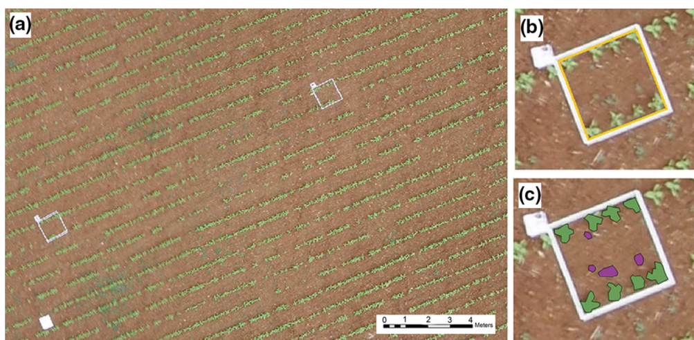
Figure 27: (a) Ortho-mosaicked imagery showing the sunflower rows and the square frames placed between two sunflower rows ; (b) Detail of vector file created for every square frame (yellow); (c) detail of the vector file created for the sunflower crop (green) and weed (violet) classes. Source: Lopez-Granados (2015).
