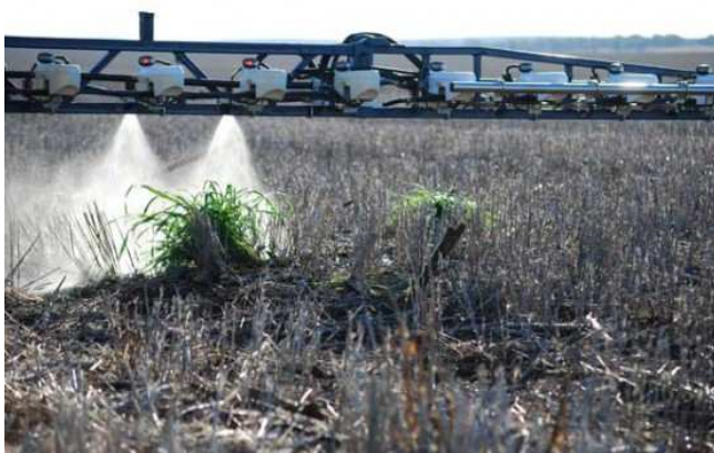
Figure 34: Real-time sensor-based VR pesticide application. Source: Southern Precision, 2016.
