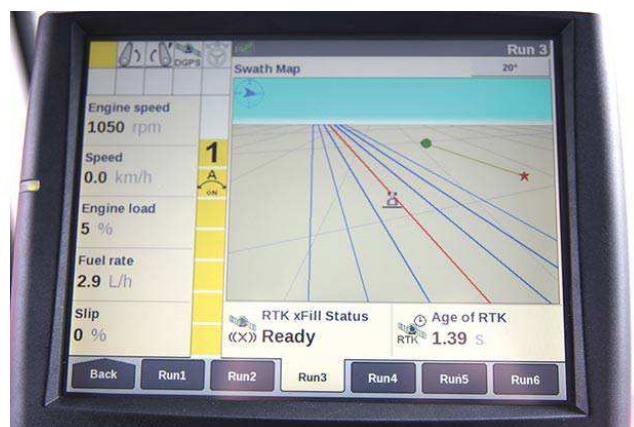
Figure 6: Board computer User Interface showing AB lines and different passes. Source: Farmers Guide, 2016.
