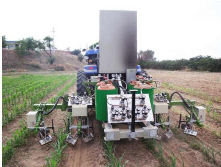
Figure 42: The hoeing-flaming implement designed by the RHEA project. Source: RHEA project, 2016.
