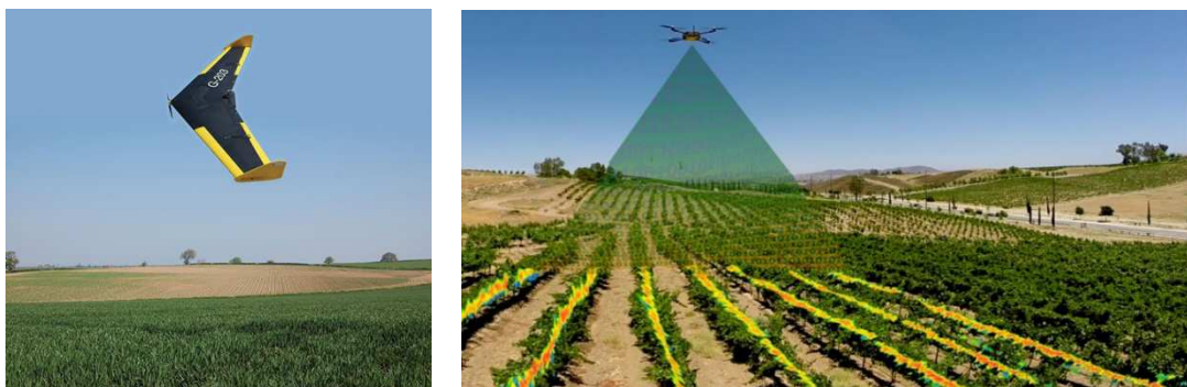
Figure 26: Fixed wing UAV (left) and rotor craft (right) UAV. Source: Farmers weekly, 2016; Nexdrone, 2016.
