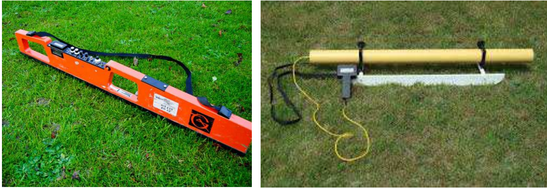
Figure 11: Geonics EM38 (left) and DUALEM 21 (right). Source: Sandberg GPR, 2016.
