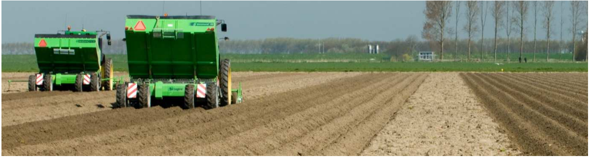
Figure 5: Machine guidance with RTK allows efficient field operations. As shown here, the planters can skip rows and filling in later thanks to precise machine guidance (photo: Jeroen Verschoore).
