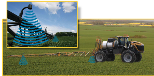
Figure 40: Boom height control. Source: GPS Ontario, 2016.
