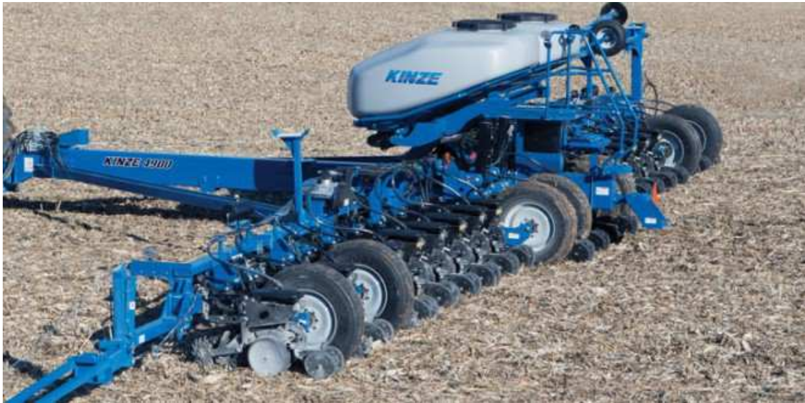
Figure 45: Multi-hybrid planting/seeder with two seed hoppers. Source: Real Agriculture, 2016.
