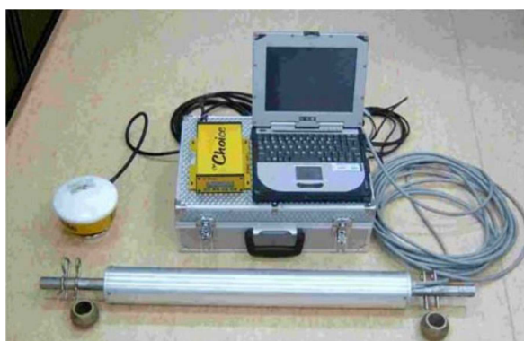
Figure15: \gamma -ray for tractor application by The Soil Company, NL. Source: Van Egmond et al., 2010.
