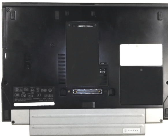
Figure 39. The installed selective laser sintered memory cover in the middle of the portable computer.
