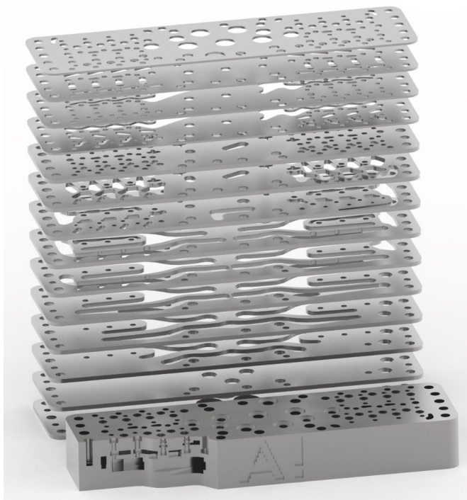
Figure 24. Original design and manufacturing method of the digital hydraulic manifold.
