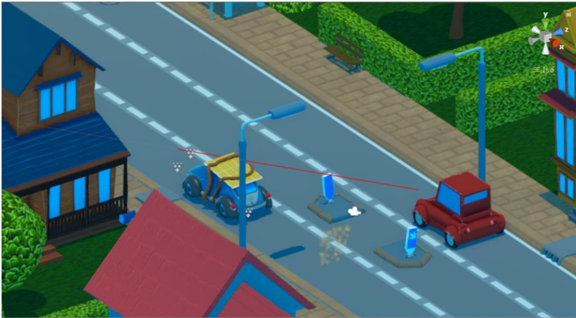
Figure 22 – Ray cast used to determine which world position is being clicked for the player
