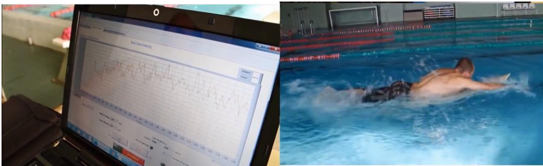
Figure AP II-1. The left image shows acquisition of velocity signal and the right image shows tests executed in the swimming pool.
