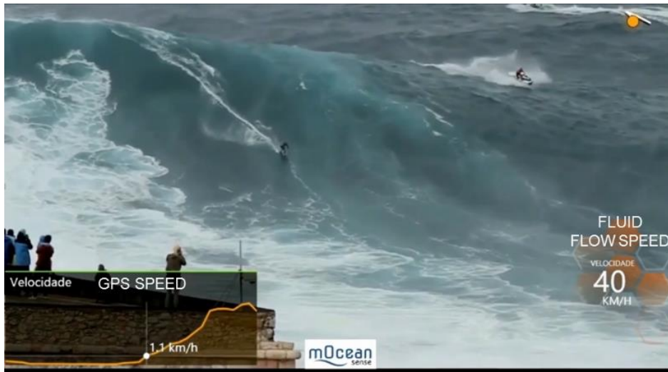
Figure 9-5 Example of GPS information showing wrong information, and our fluid flow sensor measuring the real speed.
