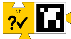
Figure 4.4: The contents of the Tactode if piece: color, text, icon, Aruco tag and indentation.
