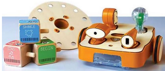
Figure 2.28: The robot KIBO and some of its tangible programming blocks.
