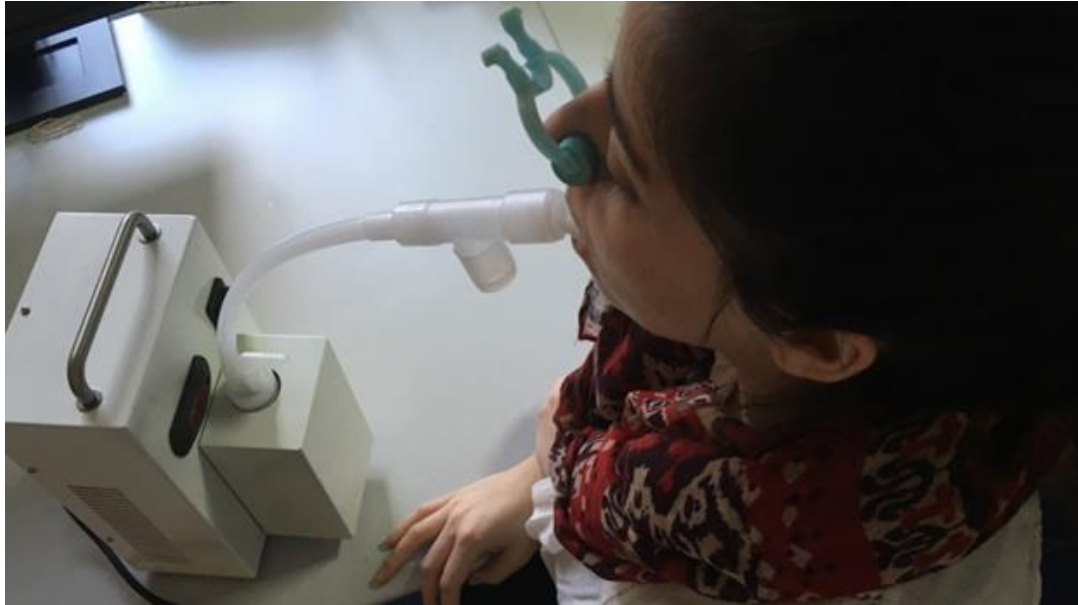
Figure 5. Collection of EBC. To collect exhaled breath condensate, children breathe normally into a mouth piece connected during 10 to 15 minutes to an exhaled air condensing system (portable Turbo DECCS).
