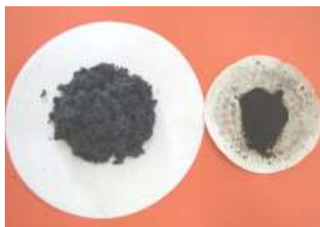
Figure 4: Effect of CaO hydrolysis on leather volume for test T3.6: initial material and dehydrated sludge
