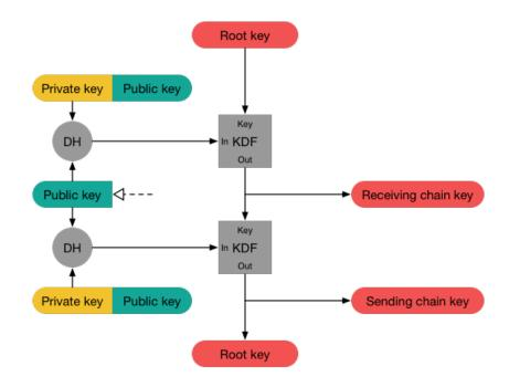
Figure 3.5: KDF chain using a symmetric-key ratchet and a DHR example [28].
