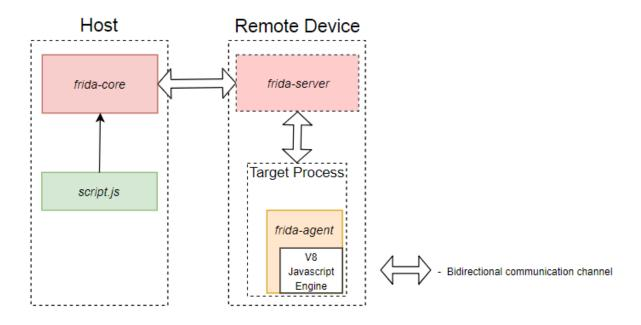
Figure 4.2: Frida componenet interaction in a remote target host scenario.
