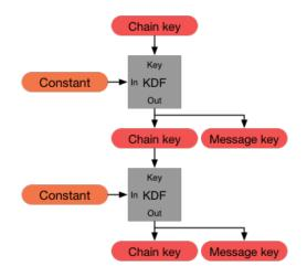
Figure 3.2: KDF chain implementing a symetric-key ratchet example [28].
