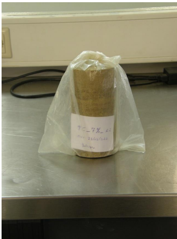
Fig. 4.14 – Specimen prepared to be stored in humid chamber
