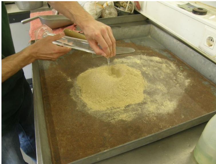
Fig. 4.7 - Specimen preparation: adding water to the soil-cement mixture
