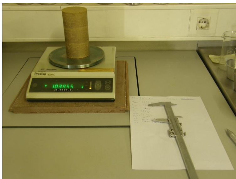
Fig. 4.13 – Weight and dimensions measurement
