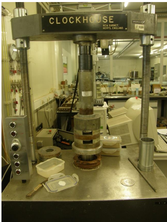
Fig. 4.11 – Specimen preparation: static compaction
