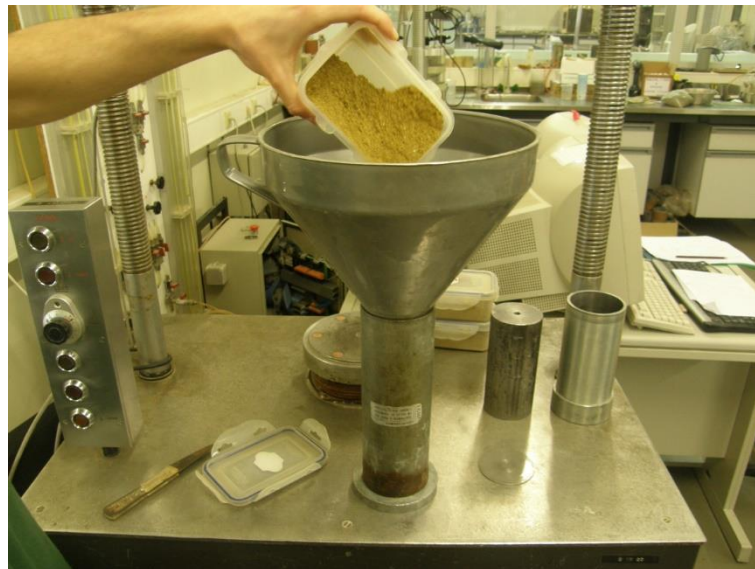
Fig. 4.10 – Specimen preparation: pouring the mixture into the mould
