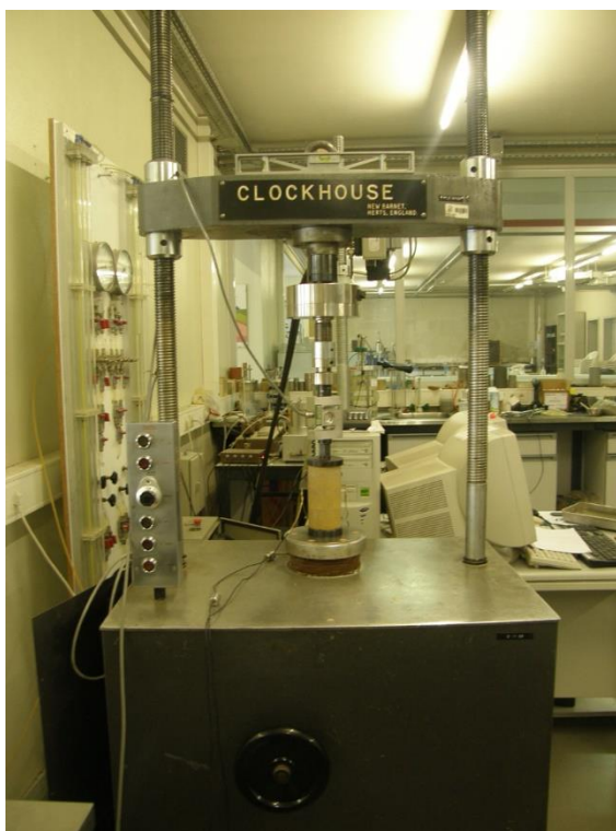
Fig. 4.23 - Equipment used for unconfined compression test
