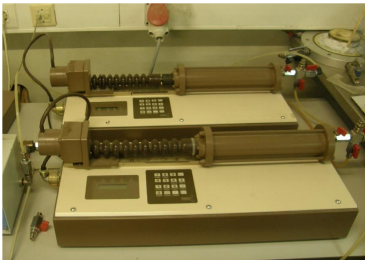
Fig. 5.6 - Digital pressure/volume controllers
