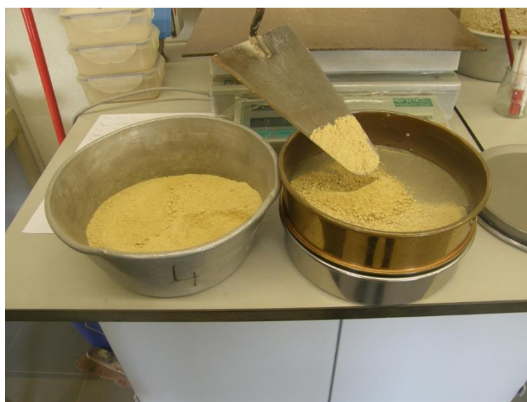
Fig. 4.4 - Specimen preparation: sieving the soil in order to remove the fine fraction
