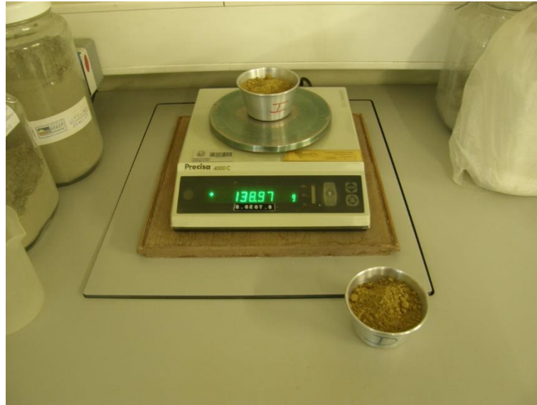
Fig. 4.9 – Specimen preparation: moisture content determination
