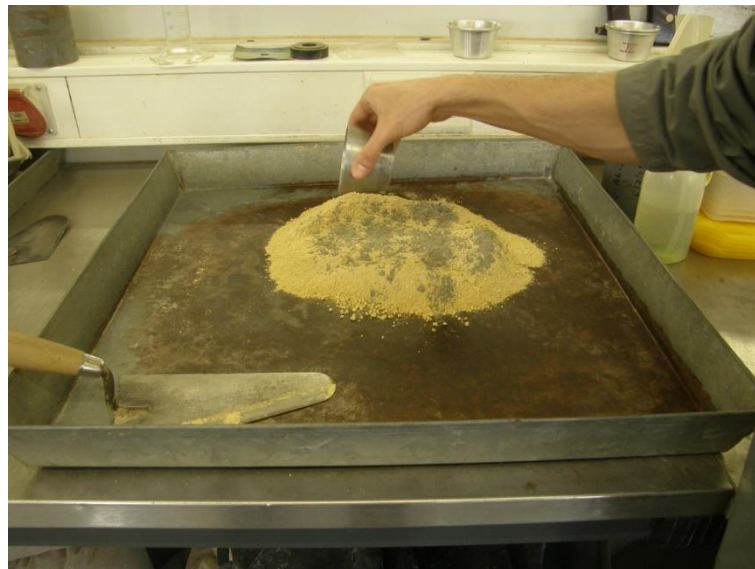
Fig. 4.6 - Specimen preparation: mixing soil and cement
