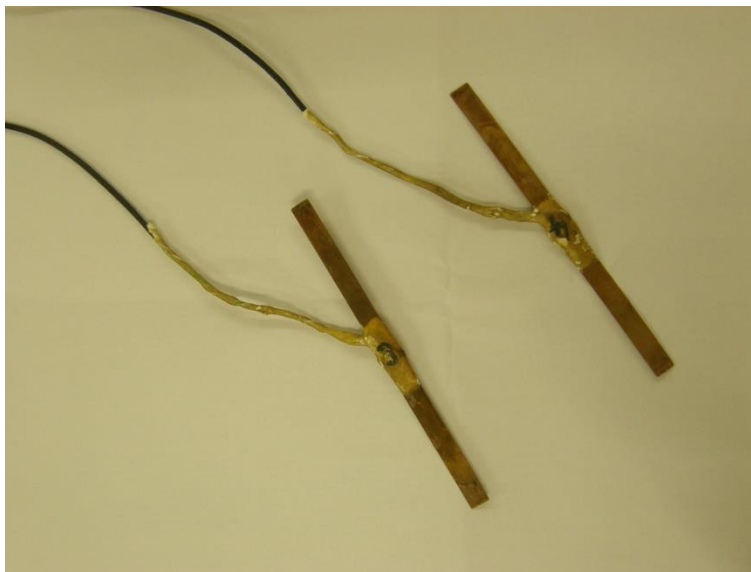
Fig. 4.24 - Two local Deformation Transducers used during unconfined compression tests
