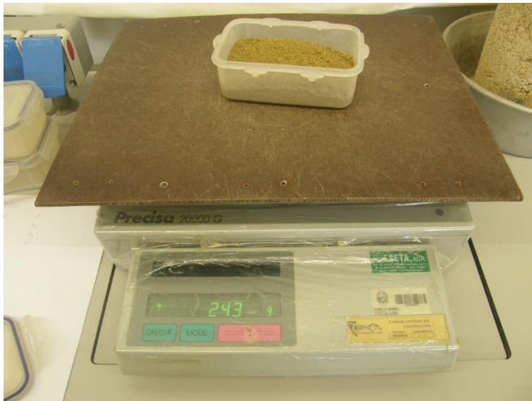
Fig. 4.8 – Specimen preparation: fractioning the mixture
