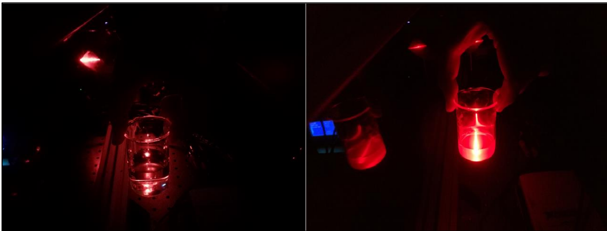
Figure 55 – Laser irradiation of (left) water solution and (right) Gd_5Si_2Ge_2 as prepared solution. The difference is clear, with more dispersion of the irradiating light in the as prepared solution.
