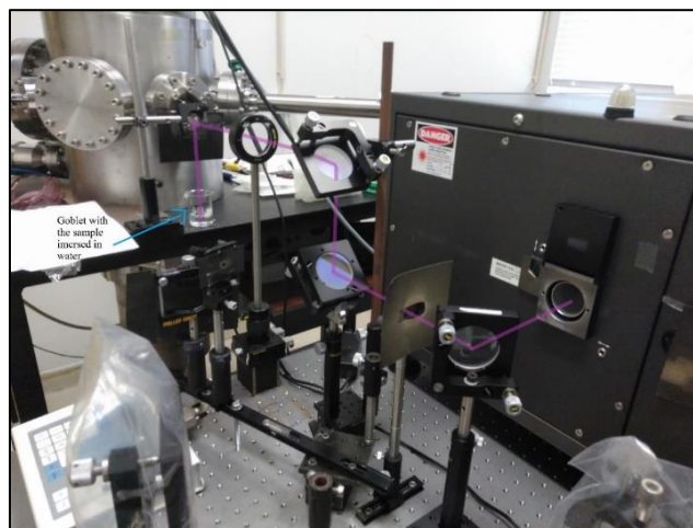
Figure 25 - Nanosecond laser ablation setup. The purple line illustrates the optical beam path. The focal distance of the lens, before the mirror (beam splitter), is of 50 cm.
