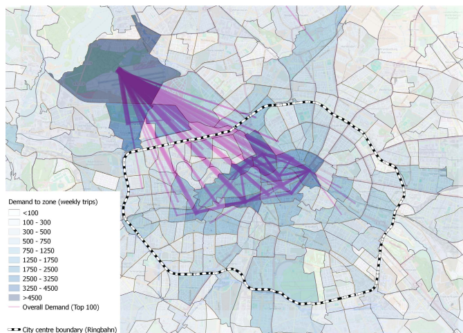
Fig. 8. Number of incoming taxi trips per zone (blue colour scale) and the top 100 OD-relations (variable-width purple lines) for the week in 2013. Map source: OpenStreetMap contributors.
