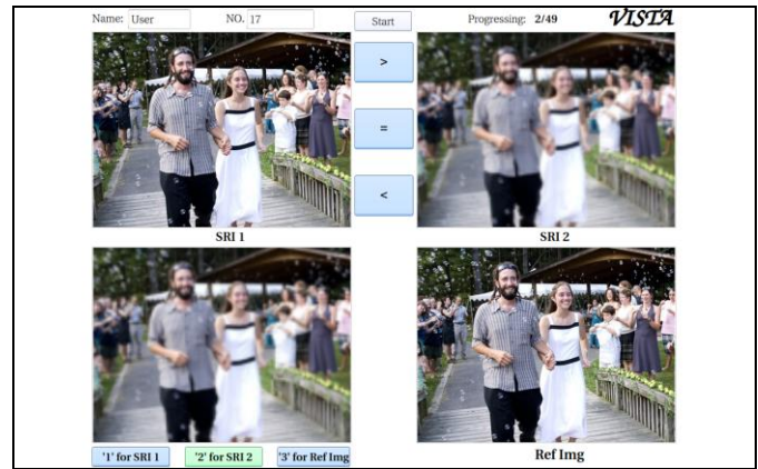
Fig. 4. Screenshot of the software interface used in subjective evaluation. The resolution of the interface is 1440×900, which is the same as that of the monitor. With this resolution, the images in the interface can be exhibited completely without scaling.
