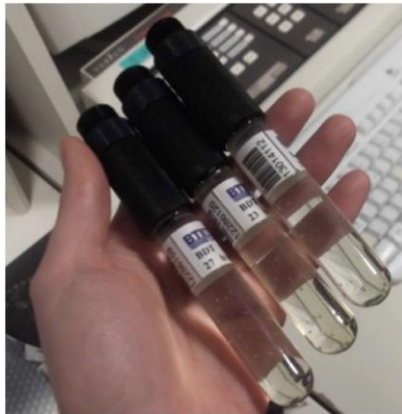
FIGURE 7.4: Bubble dosimeters representation. Neutron integral passive bubble detectors from Bubble Technology Industries (BTI).
