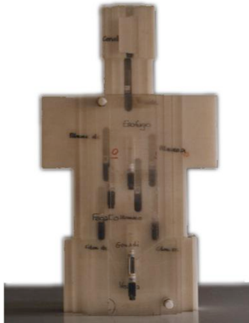
FIGURE 7.11: The Torino anthropomorphic phantom representation. Front projection. It is possible to see the holes in correspondence of critical organs with inside the BTI detectors.
