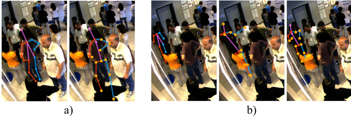
Figure 5.8: Comparison between OpenPose and Regional Multi-Person Pose Estimation (RMPE) [Fang et al., 2017]. a) and b) left show OpenPose predictions, while a) right and b) center, right show RMPE predictions. Orange joints have a confidence score below 0.2.
