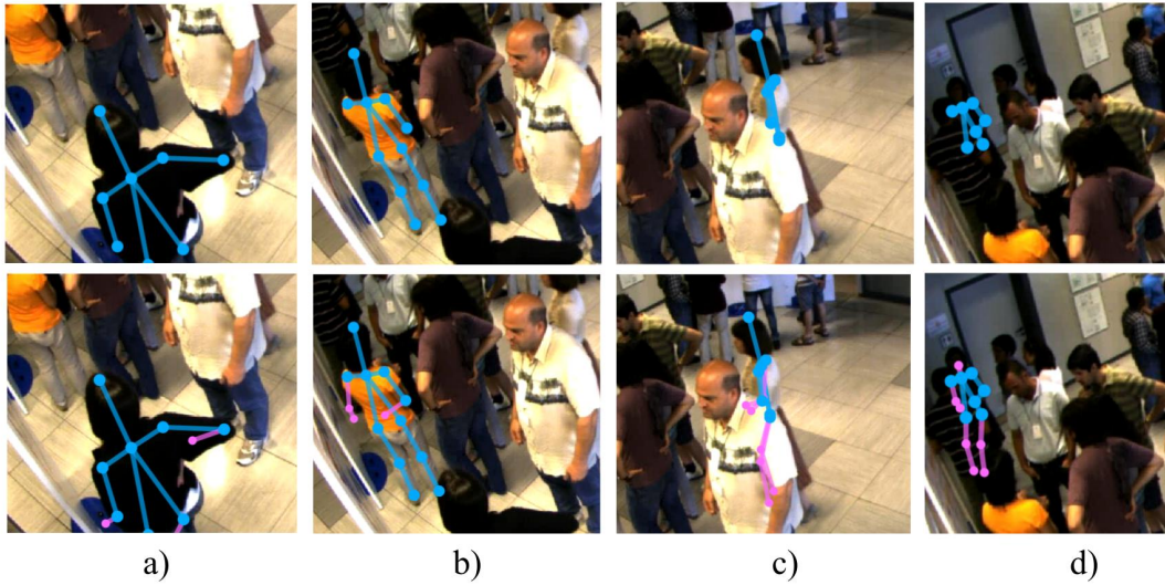
Figure 5.11: Examples of predictions on Salsa. Top row: OpenPose results (in blue). Bottom row: missing joints predicted by our method (in magenta).
