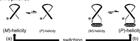
Scheme 1. Two-way control of helical-sense preferences through the intramolecular transmission of point chirality (*) associated with a dynamic helical loop in the (a) absence or (b) presence of an achiral additive.
