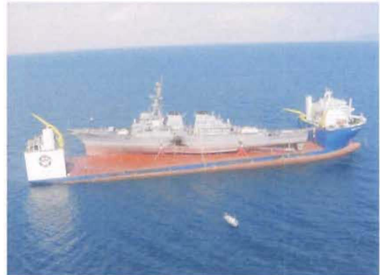
Fig. 2: Semi-submersible heavy lift ship.
