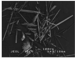
*Figure 4(b).* Purified PCA viewed at magnification of  $\times$  43
