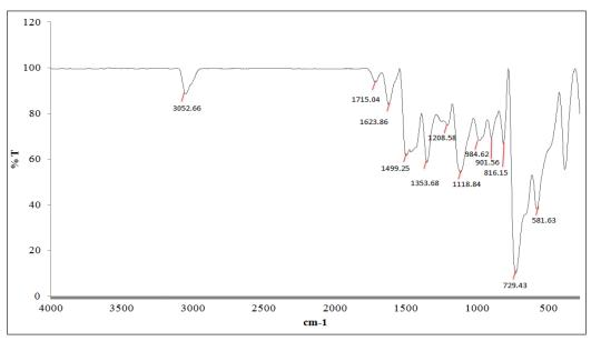
Figure 2(a). FTIR spectrum of PHZ
