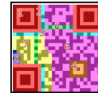
Figure 3: The structure of QR code version 2
