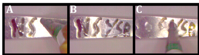
Figure 3. Writing/erasing of copper letters on a spoon, for more information, check video 1 in Supporting Information. (A) writing with copper; (B) full text; (C) copper erasing.
