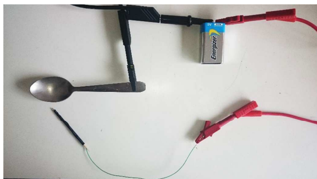
Figure 2 : spoon and electrochemical pen connected to a battery.
