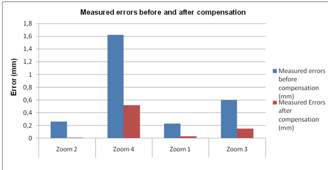
Fig. 9 Histogram of measured errors before and after compensation in the most critical areas
