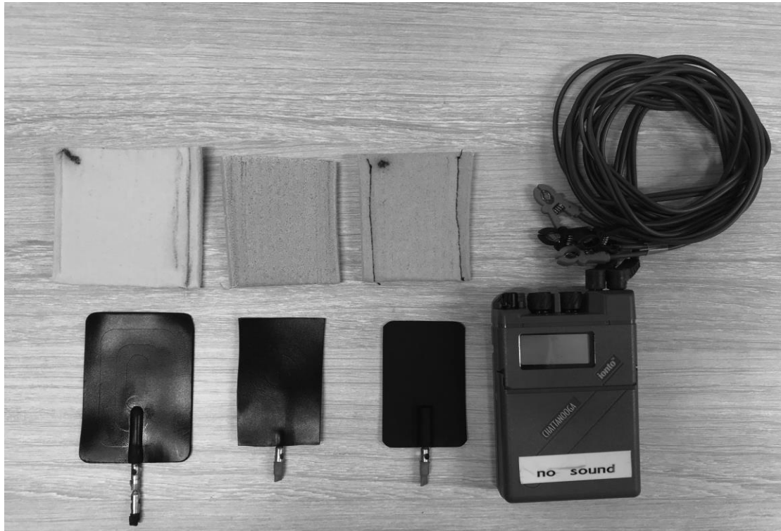
Figure 3. The tDCS was delivered using the Chattanooga Ionto™ Dual Channel Iontophoresis System. The cathode electrode (left) was inserted through 6.5 cm x 6.0 cm surface sponge electrodes and the anode electrodes (middle and right) were inserted through 5.5 cm x 4.5 cm surface sponge electrodes.
