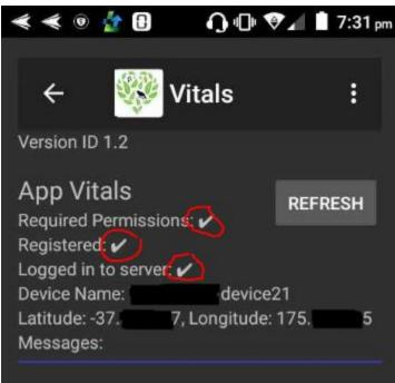
Confirm that you can see the 3 ticks and that there is a Device ID. Return to the main screen (shown below) and press the 'RECORD NOW' button to do a test recording.
