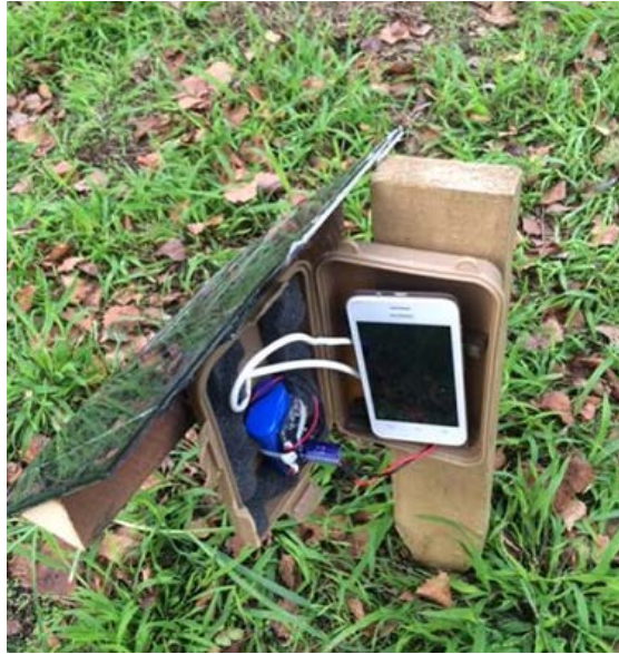
Figure 1. Cacophonometer composed of smart phone, water proof case and solar panel
