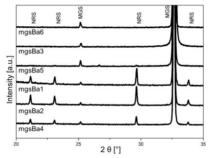
Figure 4.1-3: X-ray diffractograms of crystals retrieved from the reactors after experimental runs. Crystals of experiments mgsBa3 and mgsBa6 (Ba:Mg  $< 2 \times 10^{-4}$ ) show only peaks resulting from magnesite (MGS). In experiments mgsBa5, mgsBa1, mgsBa2 and mgsBa2 (Ba:Mg  $> 2 \times 10^{-4}$ ), norsethite reflections can be identified additionally (NRS). Unlabeled peaks stem from contamination by graphite from the stirrer inside the HMFR reactor.
