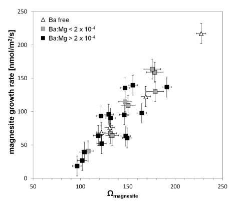
Figure 4.1-5: Growth rate of magnesite at 100 °C as a function of solution saturation state with respect to magnesite ( $\Omega_{magnesite}$ ). Growth rates show no dependence on aqueous barium concentration within analytical error.
