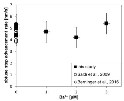
Figure 4.1-8: Obtuse step advancement rates on magnesite (104) surfaces show no dependence on aqueous Ba concentrations under the investigated experimental conditions. Velocities agree with Ba-free data by Saldi et al. (2009) and Berninger et al. (2016).
