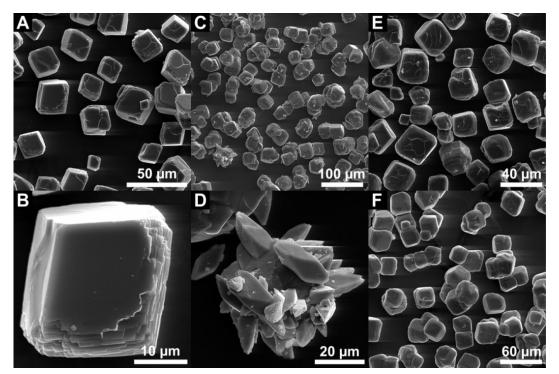
Figure 4.1-1: SEM images of magnesite crystals before (A & B) and after (C-F) experiments. C & D show crystals from experiment mgsBa1: magnesite seed crystals continued to grow (C); some magnesite crystals are covered with well crystallized norsethite needles (D), while others remained free. Experiments mgsBa6 (E) and mgsBa3b (F) yielded only magnesite
