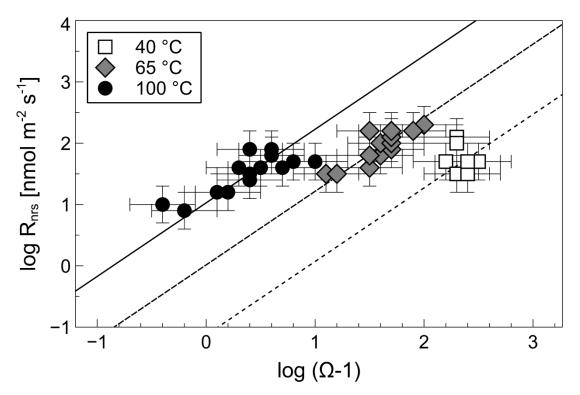
Figure 4.3-6: Logarithmic plots of measured norsethite growth rates  $R_{nrs}$  vs. supersaturation  $\Omega$  with respect to norsethite. Datasets at 40, 65 and 100 °C have been fitted to an equation of the form  $R=k(\Omega-1)^n$  with an order of reaction  $n=1.2\pm0.1$  (slope). The obtained values of the reaction constant *k* (intercept with *y*-axis) are listed in Table 4.3-3.
