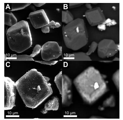
Figure 4.1-2 SEM images pairs of the same crystals after the experiments mgsBa4 (A: SE-contrast; B: BSE-contrast) and mgsBa5 (C: SE-contrast; D: BSE-contrast). Barium containing phases appear brighter in BSE contrast whereas magnesite remains dark.
