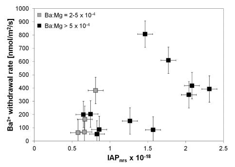
Figure 4.1-4: norsethite growth rate vs. ion activity product of norsethite. Barium withdrawal rate is equal to norsethite growth rate if norsethite precipitation is the only mechanism consuming barium. Only in experiments with  $Ba:Mg > 2 \times 10^{-4}$  norsethite was detected.
