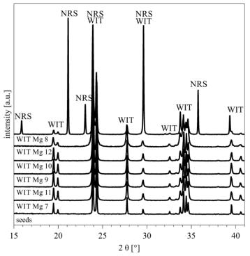
Figure 4.2-2: X-ray diffractograms of seeds and retrieved crystals. All experiments with Mg:Ba  $\leq$  6:1 yielded only witherite (WIT), except for experiment WITMg 8 (Mg:Ba > 12:1, top), which is mostly norsethite (NRS). Rietveld refinement yields a mixture of 90 wt.% norsethite and 10 wt.% witherite.
