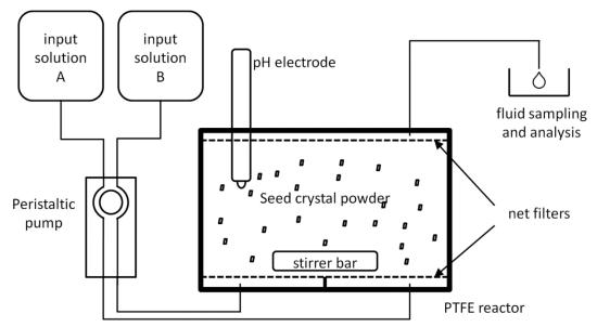
Figure 3.1-1: Experimental setup of mixed flow reactor with in-situ pH electrode. The two input solutions are mixed inside the reactor to avoid supersaturation and precipitation in the absence of seed crystals. The PTFE reactor is placed inside a water bath for constant temperature (from Lindner and Jordan, 2018).
