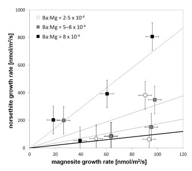
Figure 4.1-11: HMFR magnesite growth rate and norsethite growth rates are directly correlated as a function of the Ba:Mg ratios of aqueous solutions. At Ba:Mg >  $2 \times 10^{-4}$ , norsethite growth rates exceed magnesite growth rates. Thin lines are linear fits to the three datasets; the bold line has a slope of one, indicating equality of magnesite and norsethite growth rate.
