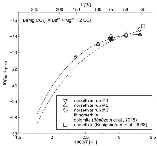
Figure 4.3-1: Logarithm of norsethite solubility product obtained in this study as a function of reciprocal temperature with the fit of the data (the uncertainties,  $\pm 0.3$ , correspond to the size of the symbol). For comparison, the 25 °C value from Königsberger et al. (1998) as well as the fit of the dolomite solubility product determined by Bénézeth et al. (2018) is reported on the plot.
