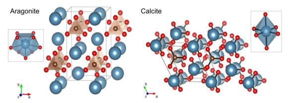
Figure 1.5-1: Crystal structures of aragonite and calcite. Blue: calcium, red: oxygen, black: carbon. Carbonate groups are indicated by triangles. Insets show Ca-coordination of the respective mineral.
