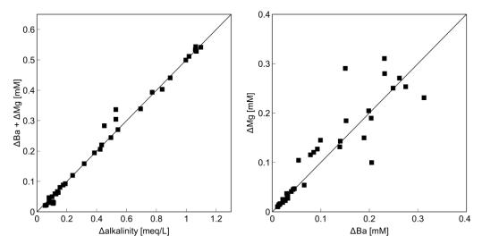
Figure 4.3-5: Mean measured concentration difference of cations ( $\Delta Ba + \Delta Mg$ ) vs. total alkalinity ( $\Delta alkalinity$ ) variation [left] and mean differences of Ba ( $\Delta Ba$ ) and Mg ( $\Delta Mg$ ) [right] between inlet and outlet fluid of the growth experiments show good charge balance and are consistent with stoichiometric norsethite growth (solid lines).
