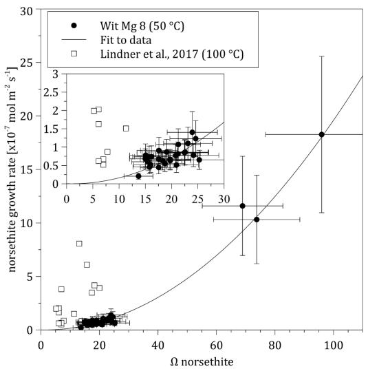
Figure 4.2-4: Norsethite growth rates vs. norsethite supersaturation. The first three samples give higher supersaturations and faster corresponding growth rates than the following samples. Rates are comparable to norsethite growth rates obtained at 100 °C (Lindner et al. 2017). The data has been fitted with an equation of the form  $R=k(\Omega-1)^n$ . For details on calculation method, see text
