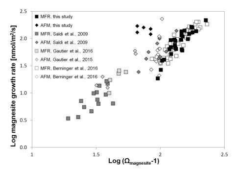
Figure 4.1-10: Compilation of magnesite growth rates at 100 °C derived from different studies. MFR: mixed flow reactor; AFM: atomic force microscopy. Note that for such comparison MFR data from Berninger et al. (2016) were recalculated using a geometrically derived seed surface area.
