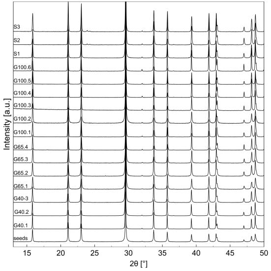
Figure Suppl1: X-ray diffractogram patterns of seed crystals and powders retrieved from the reactors after growth experiments (numbers of experiments are given) show no signs of newly precipitated phases. All major peaks can be attributed to norsethite (Ende et al., 2017). Minor amounts ( $\sim$ 1 wt. %) of witherite can be detected in the powder retrieved after solubility measurements of experiments S2 and S3, while powder from experiment S1 is free of witherite.
