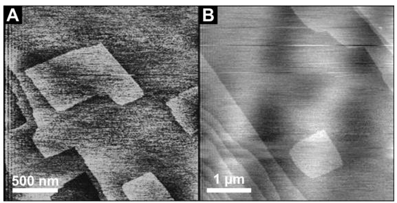
Figure 4.1-6: HAFM height images of the same (104) magnesite surface growing without (A) and with 3  $\mu$ M of Ba (B) in the growth solution (BaMg 3). The solutions are undersaturated with respect to norsethite and witherite. No influence of barium on step morphology is detectable.
