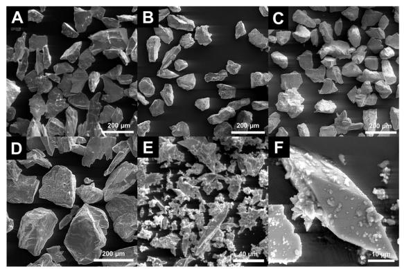
Figure 4.2-1: SEM images of crystals before (A) and after experiments without Mg (B), Mg:Ba  $\leq$  1:1 (C), and Mg:Ba  $\leq$  6:1 (D) show no difference to the used seed crystals. Mg:Ba > 12:1 (E & F) lead to dissolution of witherite and formation of many small norsethite needles.
