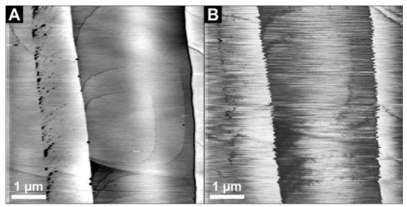
Figure 4.1-9: HAFM height images of the same surface area of experiment BaMg2 without Ba (A) and with 50  $\mu$ M of Ba (Ba:Mg  $\approx$  7 x 10<sup>-2</sup>:1) (B) in the growth solution. The presence of barium led to a significant decrease in image quality. This decrease is presumably caused by the precipitation of a Ba-carbonate phase floating within the growth solution.
