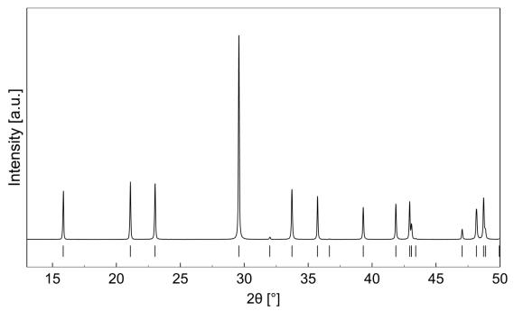
Figure 4.3-3: Exemplary X-ray diffractograms pattern of crystals retrieved from experiment G40.2 shows no signs of newly precipitated phases. All peaks can be attributed to norsethite (vertical lines, after Ende et al., 2017). The diffractograms of product powders of the other growth experiments (Figure Suppl1) do not differ significantly from the one shown.
