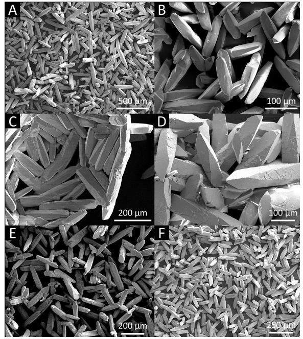
Figure 4.3-2: SEM images of norsethite seed crystals before experiments (A & B), after experiments at 40 °C (C: G40.1 & D: G40.2) and 100 °C (E: G100.1 & F: G100.6). No other phase than norsethite is discernible. Apart from an increase in size, no significant alteration of the crystals by the experiments is noticeable.
