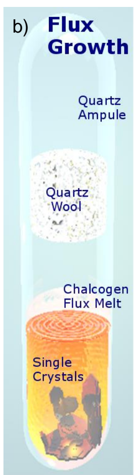
Figure 2.5: Growth Procedures for TMD Crystal Formation
