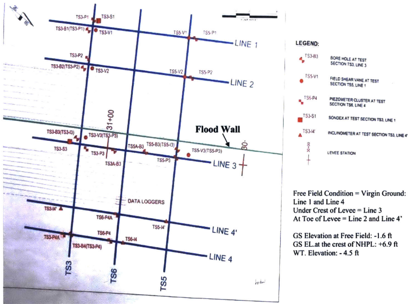
Figure 3-8: Test section area with borings, field tests and instrumentation (URS, 2003).
