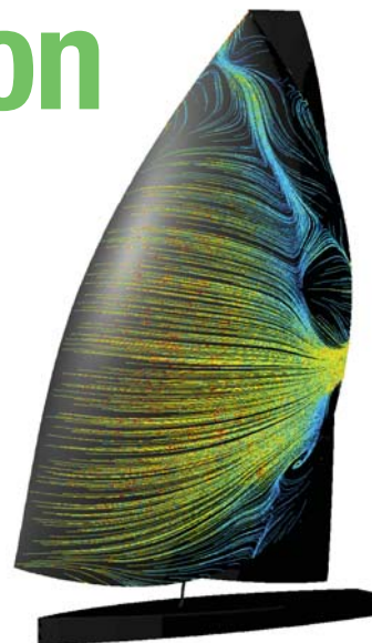
Oil-flow pathlines just above the yacht model surface. The observed tracks, colored by velocity, are painted by the wind and simulate a classic wind tunnel experiment. Converging lines show separating or re-attachment regions.
