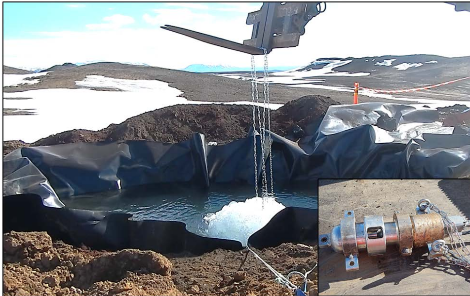
Figure 3. Water-filled zero-offset source pit with mounted air gun (lower right corner). Bubbles emerge at the water surface, shortly after source excitation.
