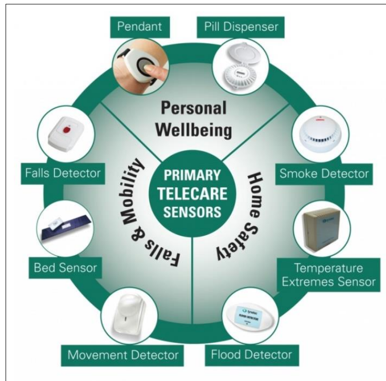
Figure 2.4 Telecare sensors wheel showing available primary sensors in Surrey (Figure taken from Surrey Telecare, 2011)
