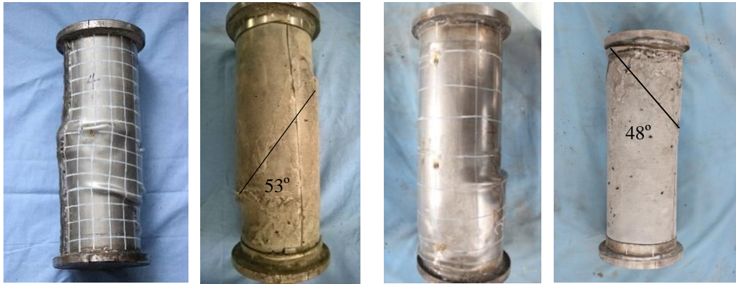
(a) Phenomena of specimen CFSST-D125-a (b) Phenomena of specimen CFSST-D150-b
