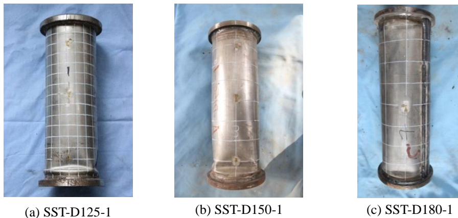
Fig.9. Experimental phenomena of stainless steel tubes with circular hollow section
