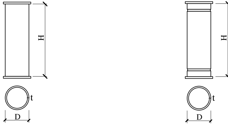
(a) Concrete filled stainless steel tube columns (b) Stainless steel tube confined concrete members
