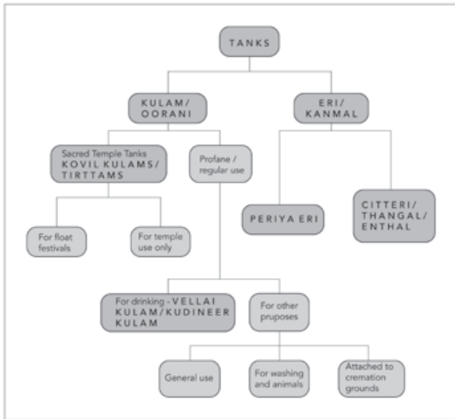
Fig.01 Classification of tanks and their names in Tamil Nadu. Vedamuthu and Rukkumany, based on Weiz (2005) and observations in the study area.
