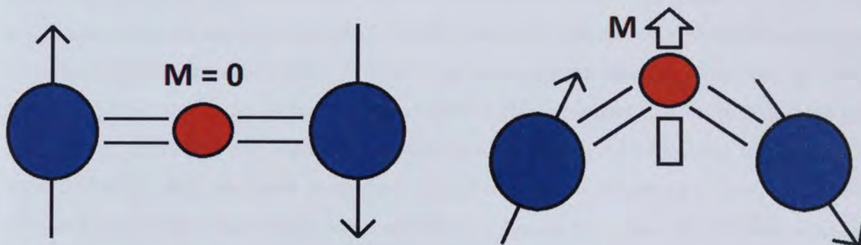
Figure 2-19 (left) Co-parallel spin structure, (right) Canted spin structure.
