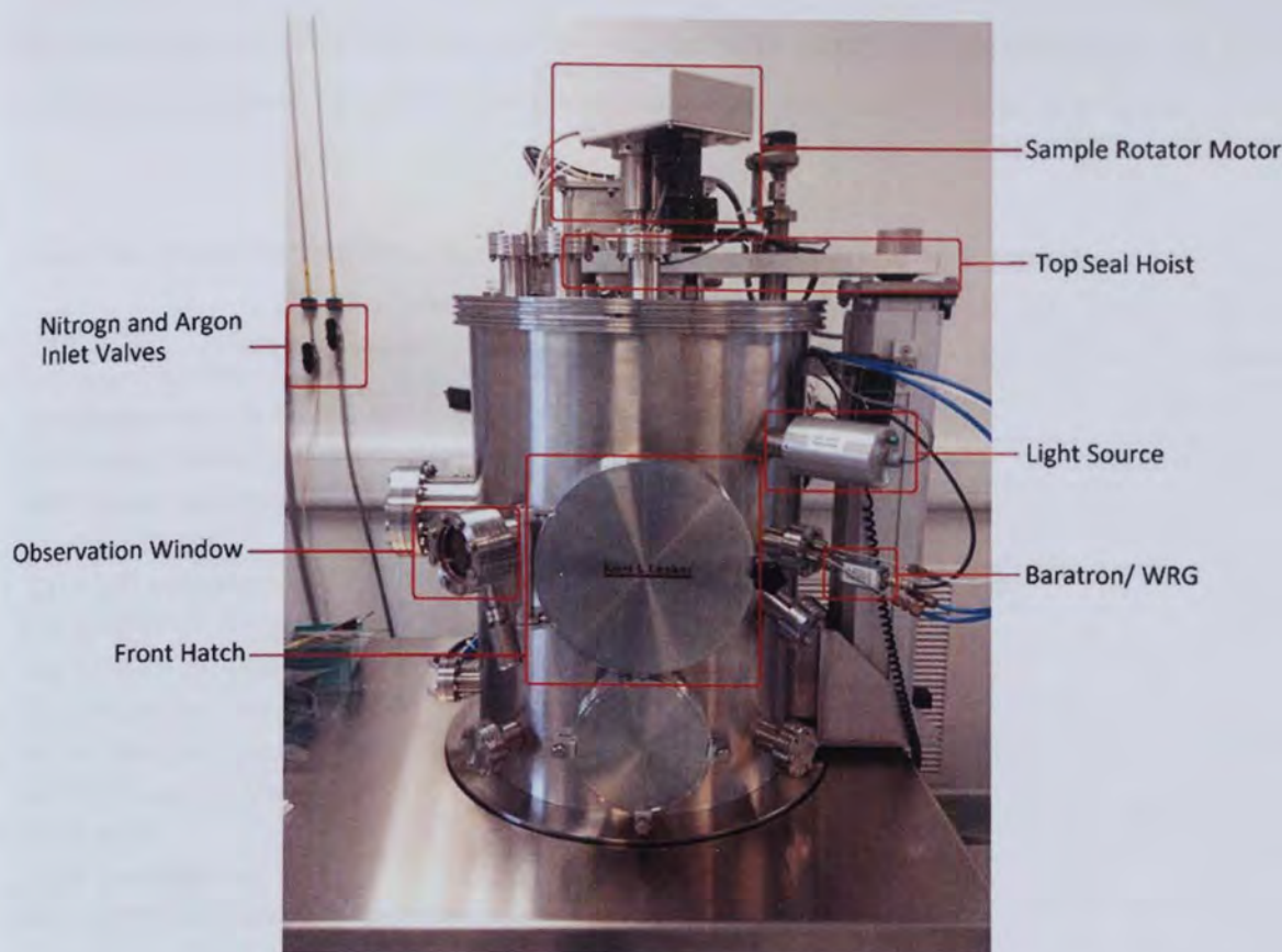
Figure 3-5 Front view of Aston Universities sputtering chamber, key parts have been labelled.
