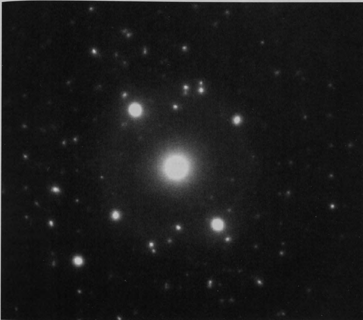
Figure 4-11 Selected Area Electron Diffraction of BTFC thin films.
