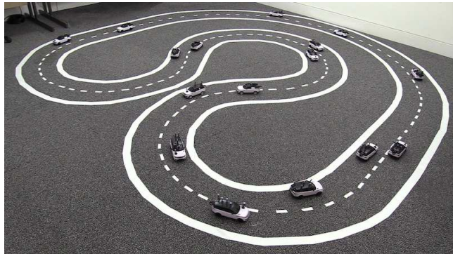
Fig. 1: The fleet of Minicars on a U-shaped two-lane miniature freeway. The inner and outer track lengths are 16 m and 17 m, respectively.
