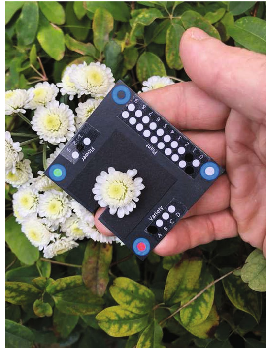
Fig. 2 An example image using a SpotCard. The SpotCard can be used at any rotation angle, allowing for easy positioning. Note the tape, to make the spots wipe-clean, and the matt black card behind the flower, reducing reflections which interfere with flower size detection
