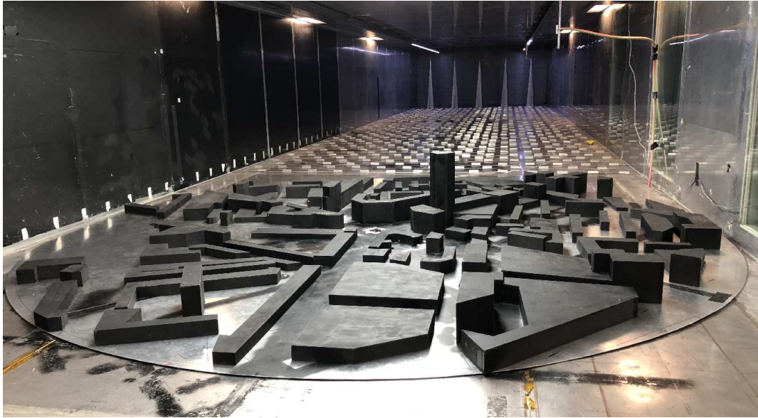
Figure 2: The photograph shows the wind tunnel model of turbulent atmospheric boundary-layer wind approaching London Southwark from the northwest.
