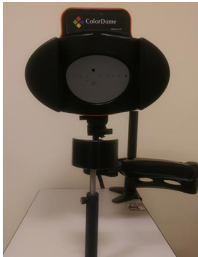
Figure 2.3. The four primary Colordome ganzfeld stimulator used to deliver the ERG stimuli.
