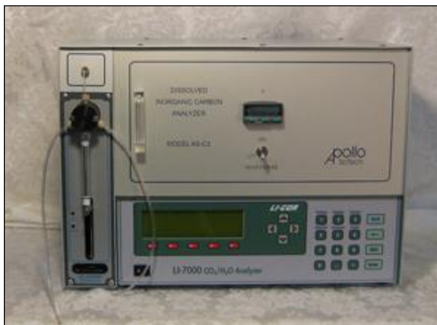
Figure 2.9 DIC analyser used for all samples during this project.
