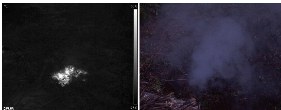
Figure 2. Experiment 3. Thermal (left) and RGB (right) image of buried fire after the hole had been closed for 1 h. Internal temperature was 250 °C, surface temperature was 77 °C. Ambient ground temperature in the area was 25–30 °C. Scale bar on the thermal image indicates temperature in °C.
