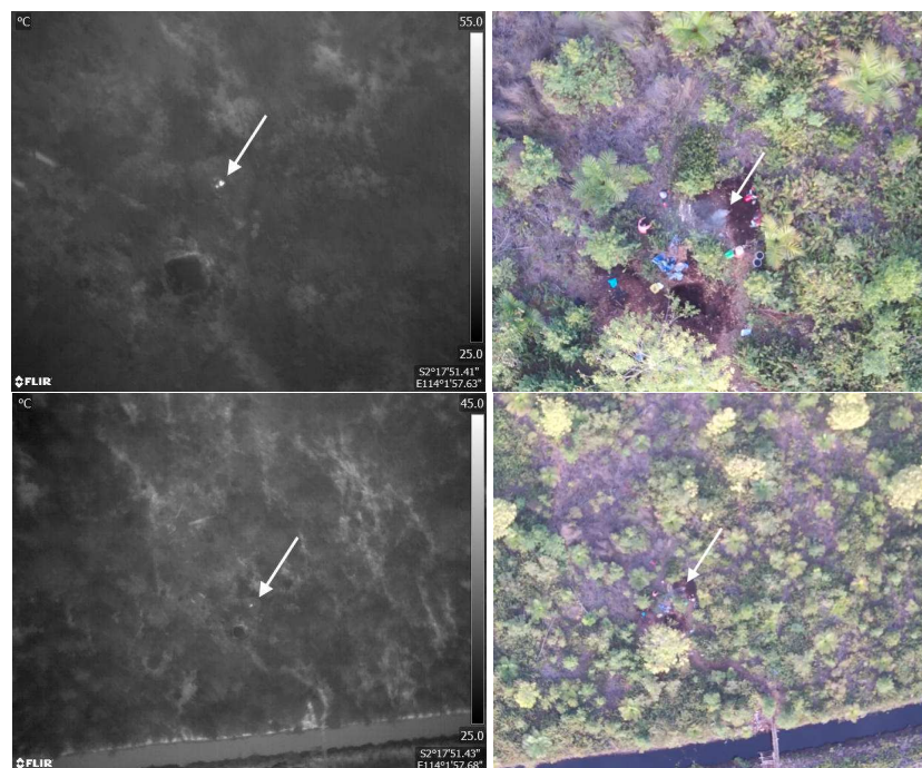
Figure 4. Experiment 5. Left: Examples of thermal data where buried fire is visible through the ground—scale bar indicates temperature in °C. Right: RGB images of same scene. Top: drone height 20 m AGL. Bottom: drone height 100 m AGL. The location of the fire as identified by the automated detection algorithm is indicated with an arrow.
