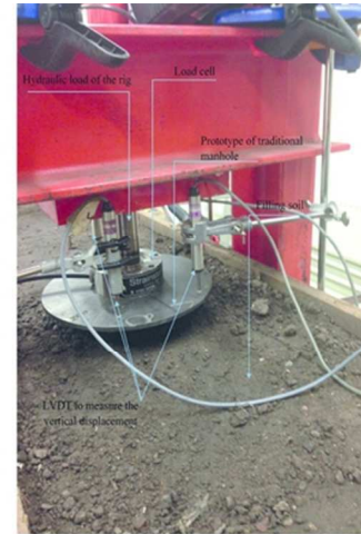
Fig. 7 b. Setup of the trench in the rig and location of measurement instruments on the traditional manhole surface at three points on the edge.
