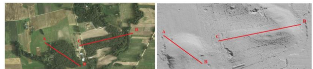
Figure 8. An example of archeological structure a) orthoimage b) terrain model generated on the basis of ALS point cloud
